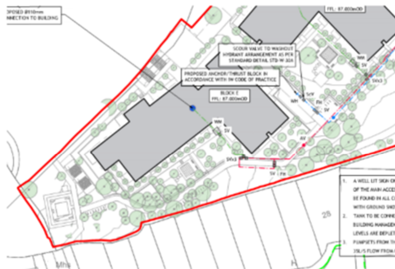
PERMITTED WATERMAIN NETWORK (refer to 192-243-021 PL1 Drainage Layout)
